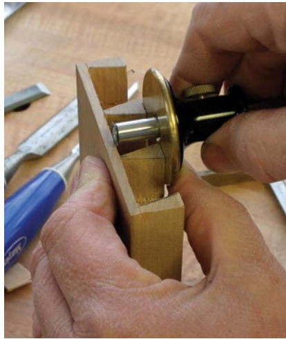
Just a cat's whisker. To accurately set your cutting gauge, allow the edge of the cutting wheel to just lip the bottom of the tail socket. Too much on the wood and your tails will be too long.
