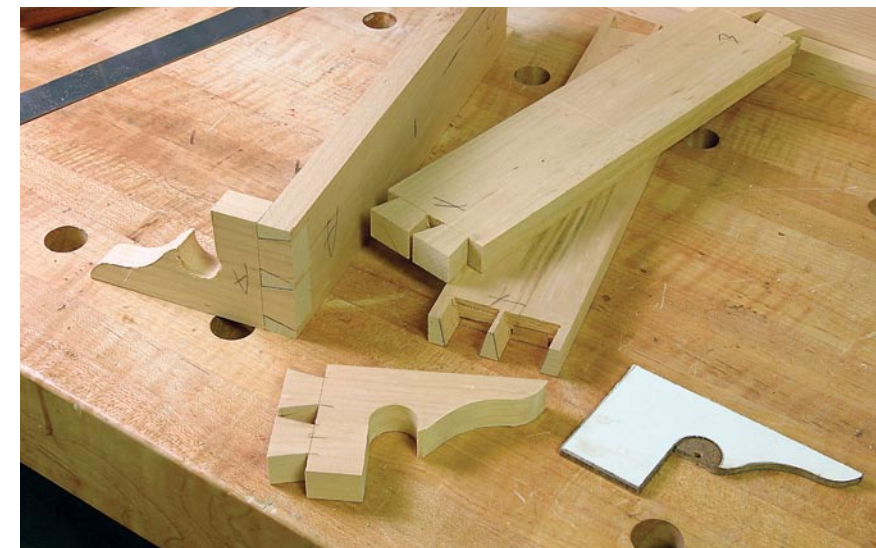
They're better paired. While scraps the length of the feet may be prevalent in your shop, working with longer pieces is easier. It also keeps the feet pins and tails matching those on the box.
