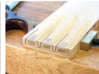
It's OK to miss this line. With the stock lying flat, make the cuts to define the pins for half-blind dovetails. Over-cutting the lines beyond the scribbleline leads to easier waste removal.
