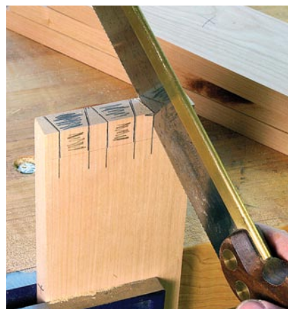
Waste side. The trick to accurate saw cuts is to follow both lines as you cut. Once you reach the scribbleline, move the saw to perpendicular and it will follow the already-cut kerf.
