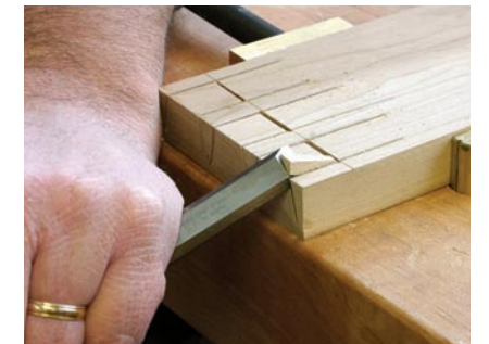
Up and at 'em. Remove small corners of waste to keep the pin corners from being fractured as you clean out the dovetail sockets.
