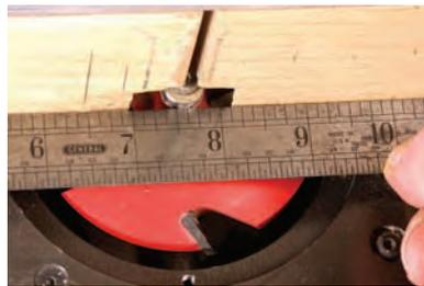
**2 Get off the fence.** For the final cut, the bearing on the cutter is flush with the face of the fence. This is a simple setting to make and return to. Get it close for now so you can make cutouts in the fence to match the cutter profile.
