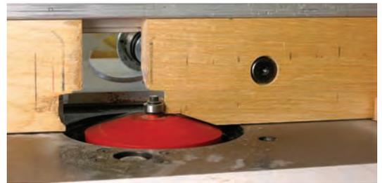
**3 Slow down and be careful.** Raised panel cutters are big so you want to minimize the amount that is exposed and slow the router down if it has a speed control. I set the router speed to its minimum and ease the sliding fences into the spinning cutter to make a zero-clearance opening. If that makes you nervous, remove the fences and cut the profile of the cutter with a jigsaw or band saw.
