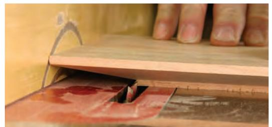
**5 Take a nip to square.** Set your fence to the measured distance plus  $\frac{1}{16}$ ", then flip the panel face down as you run four passes (one pass on each edge of the panel) over the blade to square the reveal and complete the raised panel. All that's left is sanding. You might be surprised to find out that I use power for this step as well. PW
