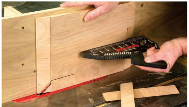
**3 Accuracy and safety.** Here you can see how the fence extension aids in making this cut safe and trouble-free. Remember to cut the end grain first. This reduces the chance of grain blow-out along the long-grain because those edges are formed last. Notice how the blade just barely peeks through the panel freeing the waste material. This is what I look for. Cut all four edges.
