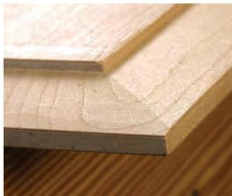
**7 Use your eyes.** Clean up the cross-grain bevells first. Then the long-grain bevells. With each pass of the plane, you'll see the bevells come into the same plane.
