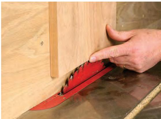
**2 Feel the blade height.** To set the height of the blade to create a raised panel, hold the panel tight to the fence extension and crank the blade up until the edge of the blade's tooth that's farthest from the fence is flush with the face of your board. That sets a  $\frac{1}{8}$ " reveal for the raise portion of the panel. Now you're ready to cut.
