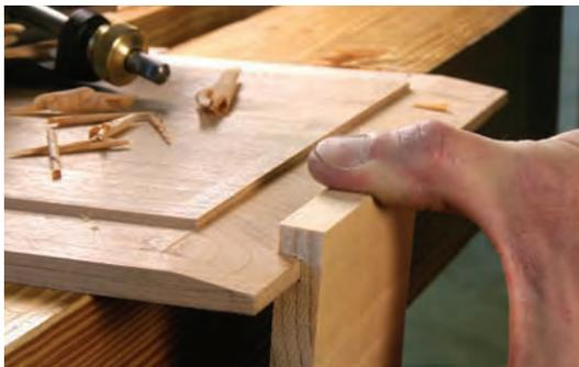
**6 Check your cut.** Use a mullet that is the depth and width of your finished groove to check the edge. When the tongue fits and the corners look good, stop planing.
