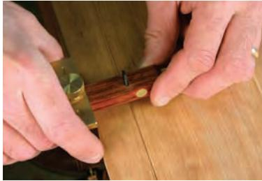
**2 Define the tongue.** Use a second cutting gauge to define the thickness of the finished tongue. Run the fence of the gauge along what will be the backside of the panel. Make this cut on all four edges.
