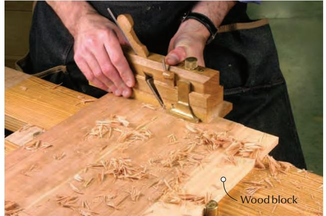
**3 First get cross.** Now sink a rabbet that is the width of your bevel and about  $\frac{1}{8}$ " deep. Work both cross-grain bevells first. Note the block of wood at the end of my stroke that prevents me from spelching the edge.
