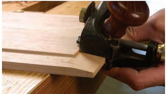
**5 Lean into it.** Now shift the fence so the tool will take a slightly wider cut—usually  $\frac{1}{8}$ " wider will do it. Why? The bevel is longer than the rabbet. Tip the plane and work the rabbet into a bevel. Work down to the line on the edge of the panel.
