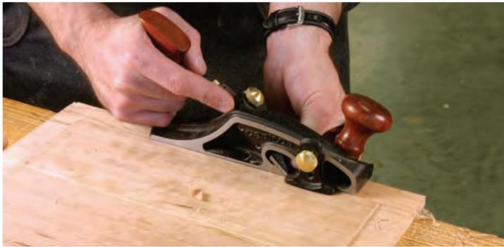
**4 Then with the grain.** Then sink the same rabbet on the long-grain sections of the panel. Don't press too hard on the fence. The skewed blade will pull the fence against the panel.
