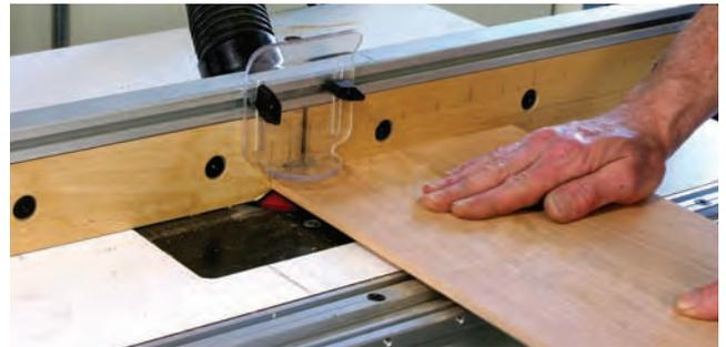
**5 Begin with the end.** Cutting across the grain can lead to tear-out as the cutter exits the wood. Make the cross-grain cuts first and the long-grain cuts that follow will clean things up. Keep the panel flat on the table and be aware of where your hands are at all times.
