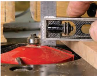
**1 Off to a good start.** There are two crucial settings to make: the height of the bit and the distance the cutter extends from the fence. I start by setting the height and use an adjustable square on top of a panel blank to leave a 1/4"-thick groove.
