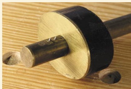
A traditional English gauge with two pins. Is it a mortise gauge or tenon gauge?
