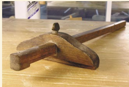
This antique panel gauge is still useful for marking out long rip cuts.
