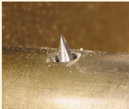
A cone-shaped pin tends to follow the grain of the wood.
