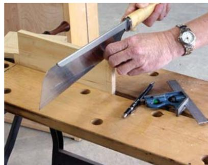
**Pinch for precision.** Just shy of your cutline, pinch with your fingers to form a guide for the cut. Slight changes in finger pressure will micro-adjust where the sawplate falls.
