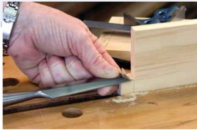
**Trim for precision.** Hold your chisel at 90° to the work and gently pare toward the shoulder to create a flat mating surface for your joint. If you need to pare the end-grain surface, take lighter cuts – and use a sharp chisel.
