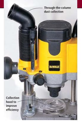
Dust collection is critical when using a hand-held router. The DeWalt has a unique collection system that pulls dust from within the base and then up through the plunge column. The Porter-Cable router also pulls dust through the base, but the vacuum port is on the base itself.
