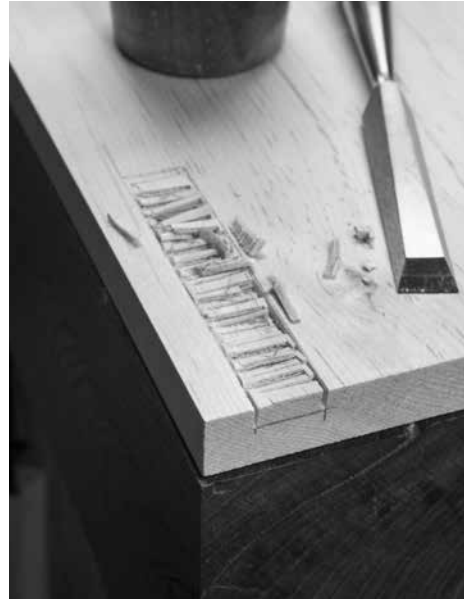
Chiseled features. You can simply chop out most of the waste with a chisel, working across the grain for the most part. Be careful if you decide to chop parallel to the grain because you could split the entire case side.
