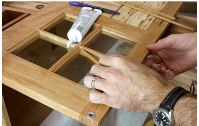
Once everything is finished, install the glass using small strips of cherry (1/8" and 1/4" thick). A few dabs of clear silicone and a couple small pins do the trick.
