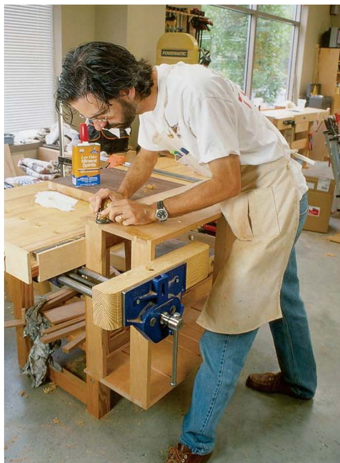
After gluing the sides to the bottom and top rails, trim the dovetails flush with a block plane. Soak the end grain with a little bit of mineral spirits to make it easier to cut. Here you can also see how I supported the case as I worked on it. The big slab holding up the side is an offcut from an old door that's clamped to my bench.
