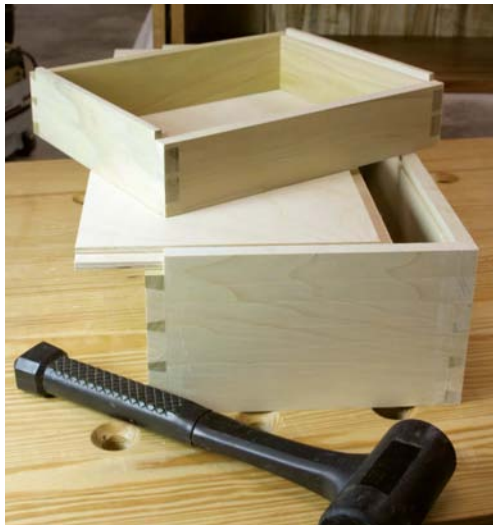
Here you can see the two different ways of installing the drawer bottoms. The bottom in the top drawer rests in a rabbet in the sides. The drawer bottom for the larger drawers slides into a groove.
