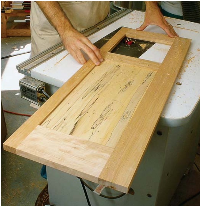
Cut the rabbet on the backside of the door using a rabbeting bit in your router table. With a large tabletop such as this, it's simple work.
