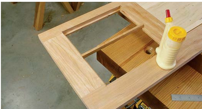
Glue one backing strip into the rabbet in the door on edge. Then flip the door over and glue a mullion onto the backing strip. Then use spring clamps to hold everything while the glue dries.
