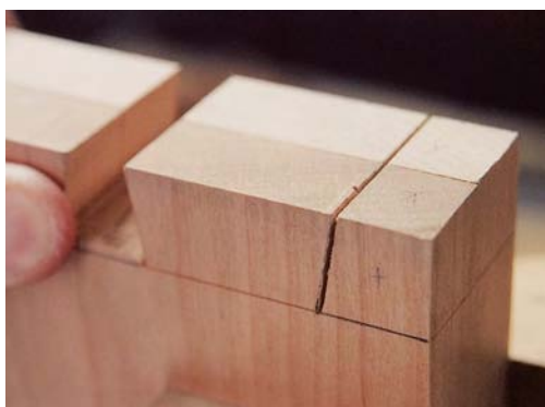
When sawing the tails, clamp the two sides together and cut them at the same time. This saves time and effort and prevents layout errors.
