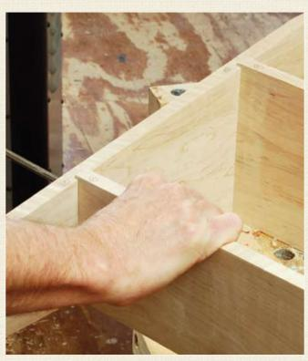
20 I then planed the bevel on each of the top two shelves and the rounded edge on the bottom shelf.
