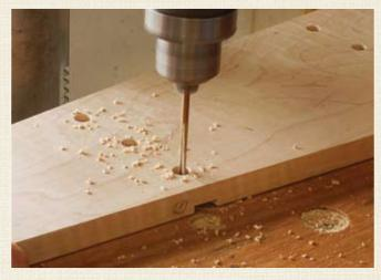
17 Then, in the center of each countersink hole, I drilled the through hole for the screws that would hold the shelf unit together. This bit is just a little larger in diameter than the threads on the drywall screws\* I would be using at assembly.
