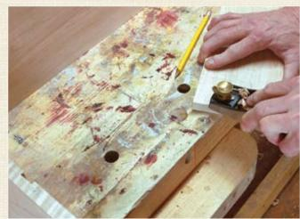
15 I cut the dadoes to a width slightly less than the thickness of the shelves, which gave me some thickness I could remove with a plane to fit each shelf to its dado.
