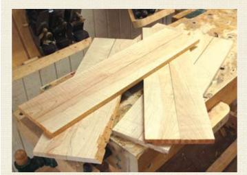
7 I began the jointing process at my machine jointer which established an edge exactly 90° from the face.
