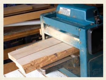
2 One option, which I frequently exercise in the case of particularly fine, wide boards, is the use of hand planes, but there is another way to handle such material: Saw it in half and after surfacing it, rejoin the halves.
