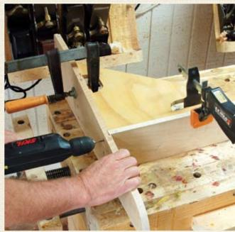
18 While its true the screws turned into end grain lack the holding power of screws turned into side grain, if you're careful to select a bit of the right size—one that allows the threads to bite into the sides of hole without requiring so much torque that they're twisted off—the screws still provide an acceptable amount of grip, particularly if you use several screws as I did.
