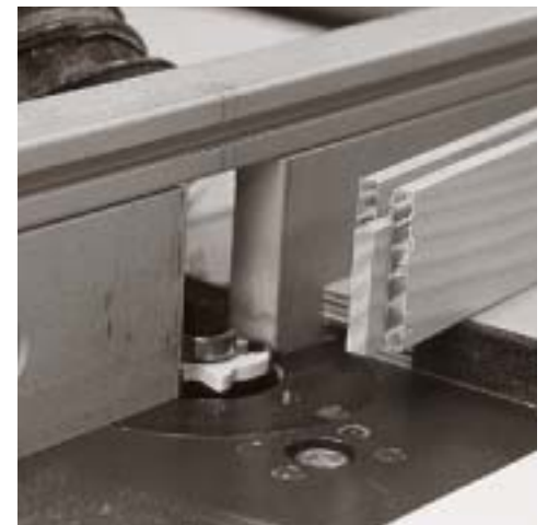
Three simple passes over a spline-cutting bit form the completed stub tenon and panel groove.
