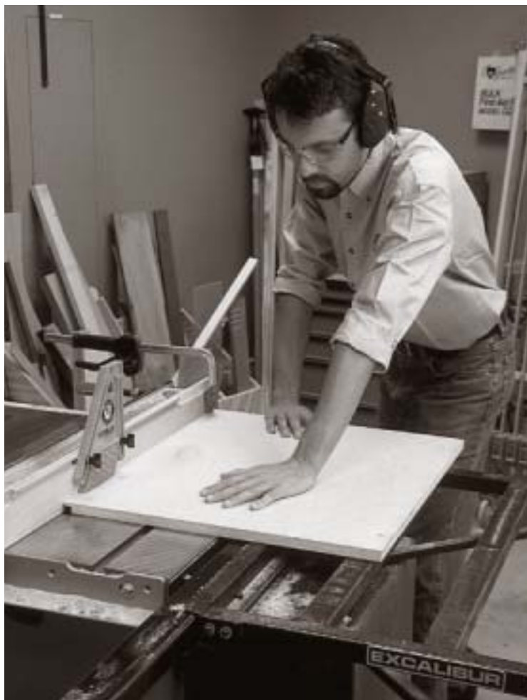
The same rules for ripping and crosscutting apply to rabbeting. For ripping cuts with the grain, use the fence to guide your cut.
