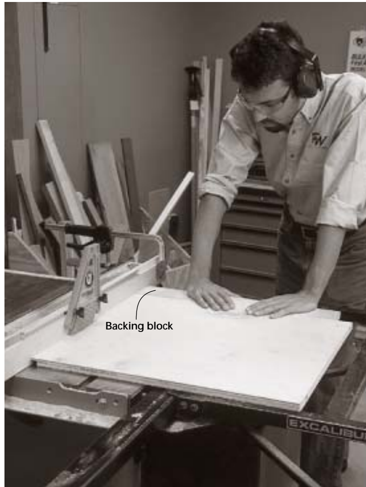
For crosscutting across the grain, use the miter gauge for narrow pieces or use the rip fence and a backing block (to prevent tear-out) for larger pieces.
