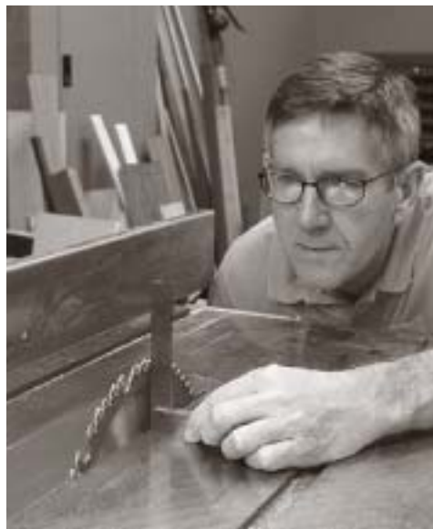
Every step of making stub-tenon doors requires square cuts, whether on the table saw or router.
