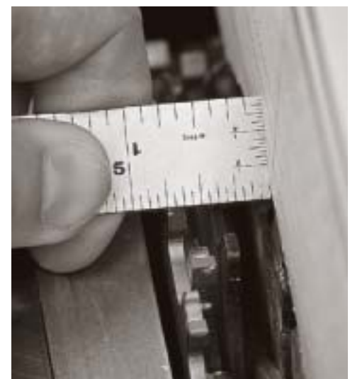
The distance from the top of the left tooth to the fence determines the width. This is ¾".
