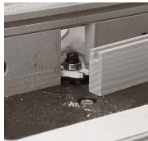
After making test cuts for the groove location, run grooves on the inside edges of all parts. It's important to keep the parts organized and marked so that the good face is up. By doing this, you'll minimize any problems caused by minor inaccuracies in centering the groove precisely.
