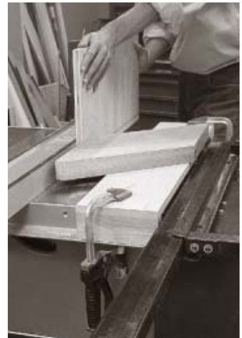
The “motherboard” keeps everything in place during the second pass. The result is a clean and accurate rabbet.
