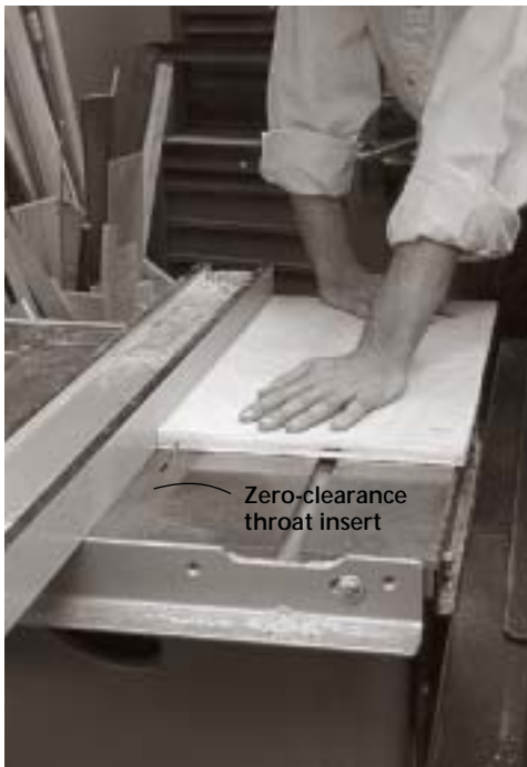
When making the cut in two stages, the first cut defines both the width and depth of your joint. Keep your work tight against the fence.
