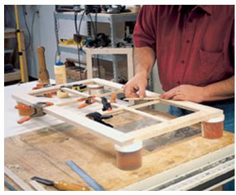
Finally, flip the door face up one more time and cut and install the remainder of the face pieces. You can install all the pieces at one time, without allowing each piece to dry. You're limited only by the number of clamps you own, but don't work so fast that things get sloppy. **PW**
