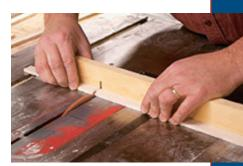
The divider pieces for these doors are made from two different sizes of wood strips. The face material is  ${}^{1}\!/{}^{4}$ " x  ${}^{3}\!/{}^{4}$ ", while the backer pieces are  ${}^{1}\!/{}^{4}$ " x  ${}^{1}\!/{}^{2}$ ". I use a new sacrificial fence on my miter gauge for each new door project to keep tear-out on the backside of the pieces to a minimum. This also makes locating the cut easier by aligning the strips with the initial kerf in the fence.
