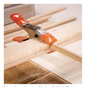
To begin the muntin section of the doors, find the shelf locations on your project's case (generally the glass dividers align with the shelves) and mark these on the edges of the door. Cut the backer material to run from side to side. These pieces divide the glass area horizontally. The fit should be snug, but not so tight as to bow the frame. Glue the backer piece into the rabbet area and clamp until dry, usually about 30 minutes.
