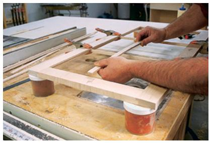
Now flip the door over. The first face pieces to install are the pieces that run the full length, in this case the center piece that divides the glass area vertically into two sections, left and right. The piece again needs to be snug, but not too tight. Glue each end (as well as each area) where the face crosses the backers (two locations in this case). You'll notice that I have the door elevated on some jars. The contents aren't important, but the elevation is very helpful.
