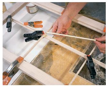
Flip the door over again and begin to cut and install the three backer pieces that complete the "T" for the glass and run from muntin to muntin. These pieces back the face piece. Glue and clamp until dry.
