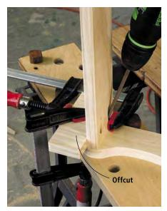
An offcut makes a handy clamping block to help you keep the shelves in place as you drive the pocket screws.
