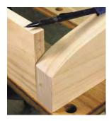
drill your pocket holes using the bit provided in the kit. For the best result, keep the angle of your drill in line with the angle of the hole, and squeeze the trigger while the bit is at the top of the hole to allow it to get up to speed before making contact with the wood. Now drill the remaining 15 pocket holes.
