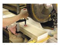
Clamp up your three side pieces (one is an extra) being sure to align the long edges as much as possible. Then, trim the ends flush.
