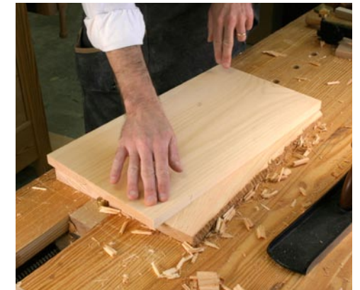
Use one flat panel to check another. If your bench is truly flat, you also can use that as a reference surface. However, a freshly flattened board is likely the more reliable barometer.
