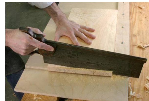
Cut the panels to length using a sash saw, then clean up the results with a plane. I use my shooting board for both operations.
