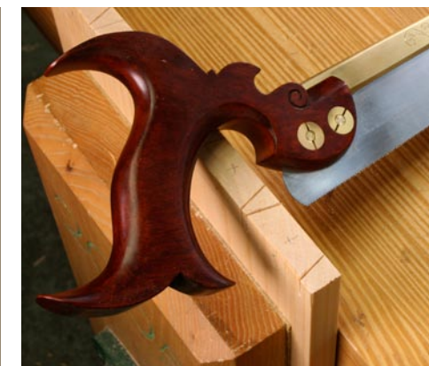
Mark the pins out with a pencil (or a knife if you please). Saw down to the baseline.
