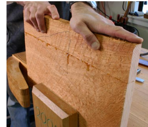
A “rub joint” is easy to execute in short panels such as needed for the school box. It’s surprisingly easy to do. Use enough pressure to close the joint, but not so much that all the glue squeezes out.
