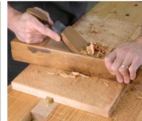
Use strokes across the grain to remove the material. Then use diagonal strokes across the panel to get the board as flat as you can. Small softwood boards are easy to process this way.
