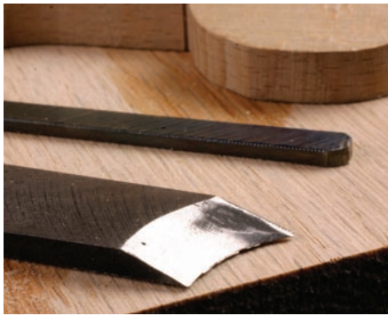
No small taper. Here you can see the bevel and the tang of two unfinished irons for snipes bills planes. The irons start thicker at the bevel and taper 1/16" along their length. That's a lot of metal work.
