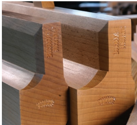
A steady hand. The swooping gouge cuts on the shoulders of the moulding planes require sharp tools and skill.
