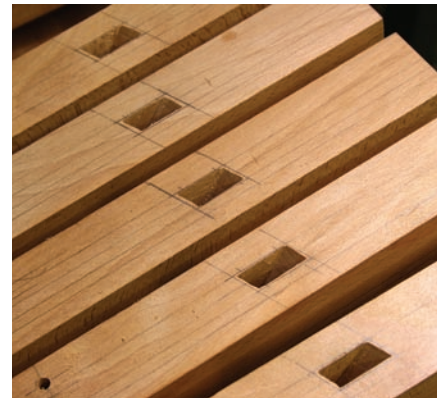
Mortises for wedges. "We've been careful not to design our tools around our machines." — Larry Williams
