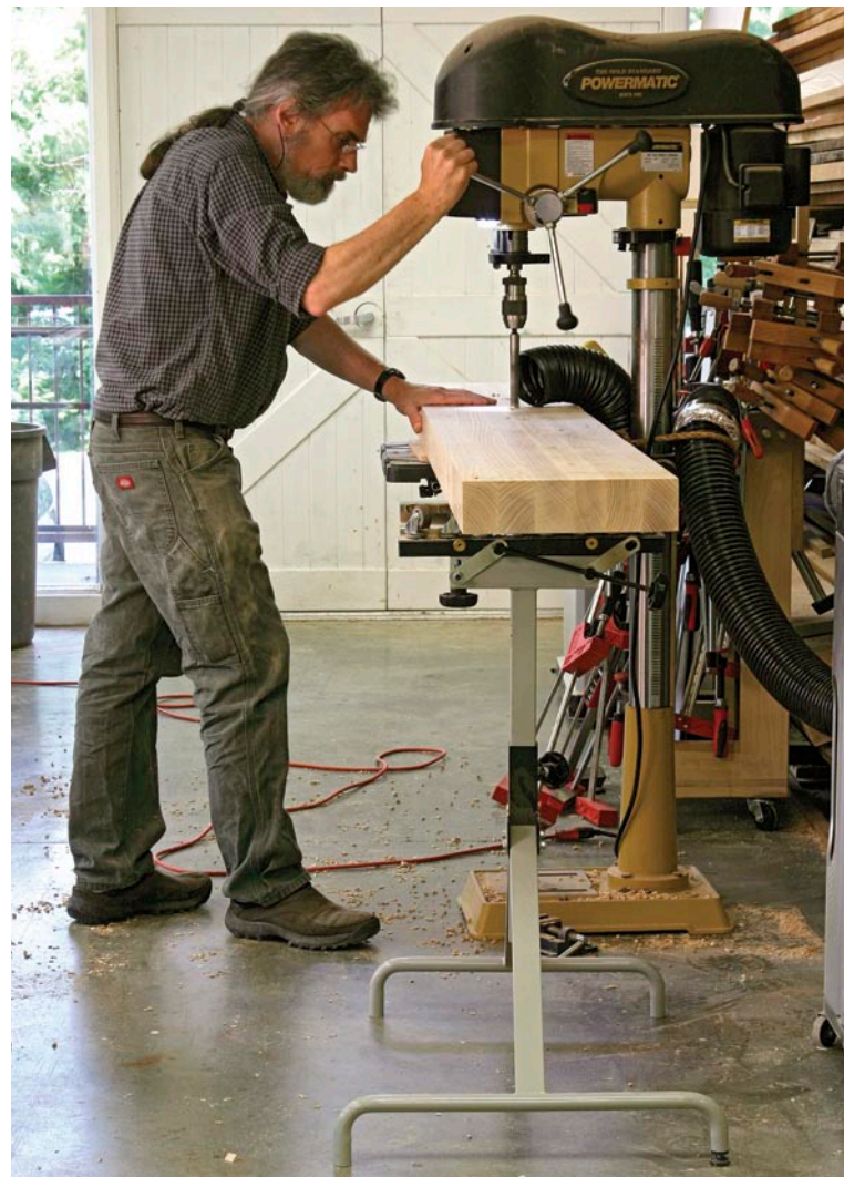
The boring part. The top halves are heavy, but with the aid of a stand they can be brought to the drill press for boring the dog and holdfast holes.
