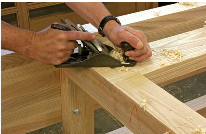
Fine-tuning. The lag bolts that secure the upper rails are counterbored to keep the heads well below the surface. The faces of the rails are made flush to the legs.
