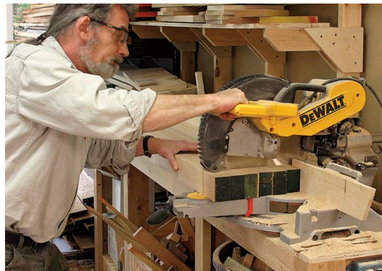
It just fits. Trimming the top halves to final length is within the capacity of this 12" sliding compound miter saw.
