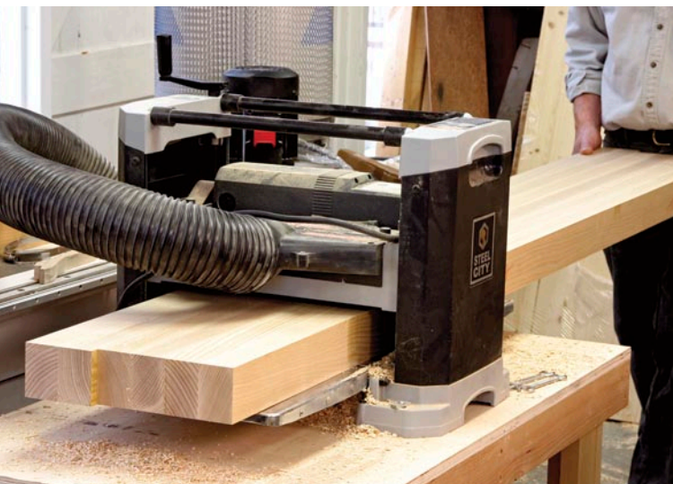
Power lunch. This bench was designed around available machinery. After cleaning one surface with a handplane, the opposite surface is planed on a portable machine.
