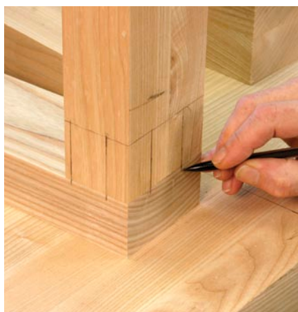
Minimize the layout. After laying out the tenon locations on the stretchers, lines are transferred to mark the matching mortises on the inner parts of the legs.
