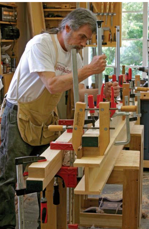
Sum of its parts. The flatness of the finished benchtop depends on the quality of its component parts. Milling the pieces as true as possible and gluing them together on a flat surface is crucial.
