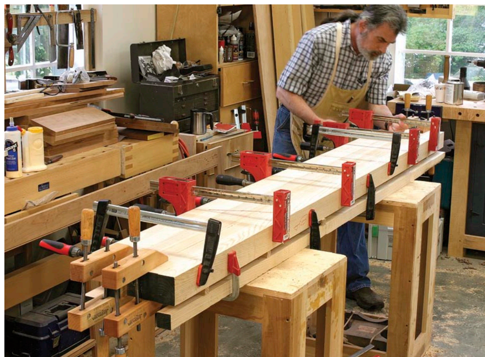
Practice makes perfect. Taking time to set up a level and accessible surface for gluing, and making a dry run, makes the final glue-up stress-free and yields good results.
