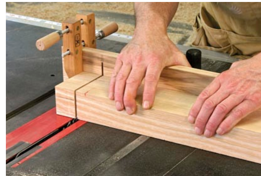
Tenons, plan B. The tenons can also be cut on the table saw, but the machine must be adjusted several times to hit the layout lines precisely.
