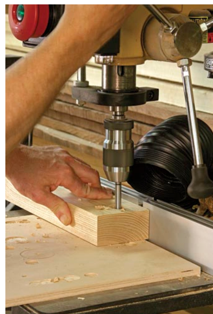
Wasting away. A 3/4" Forstner bit in the drill press is used to remove most of the material from the through-mortises in the inner legs.
