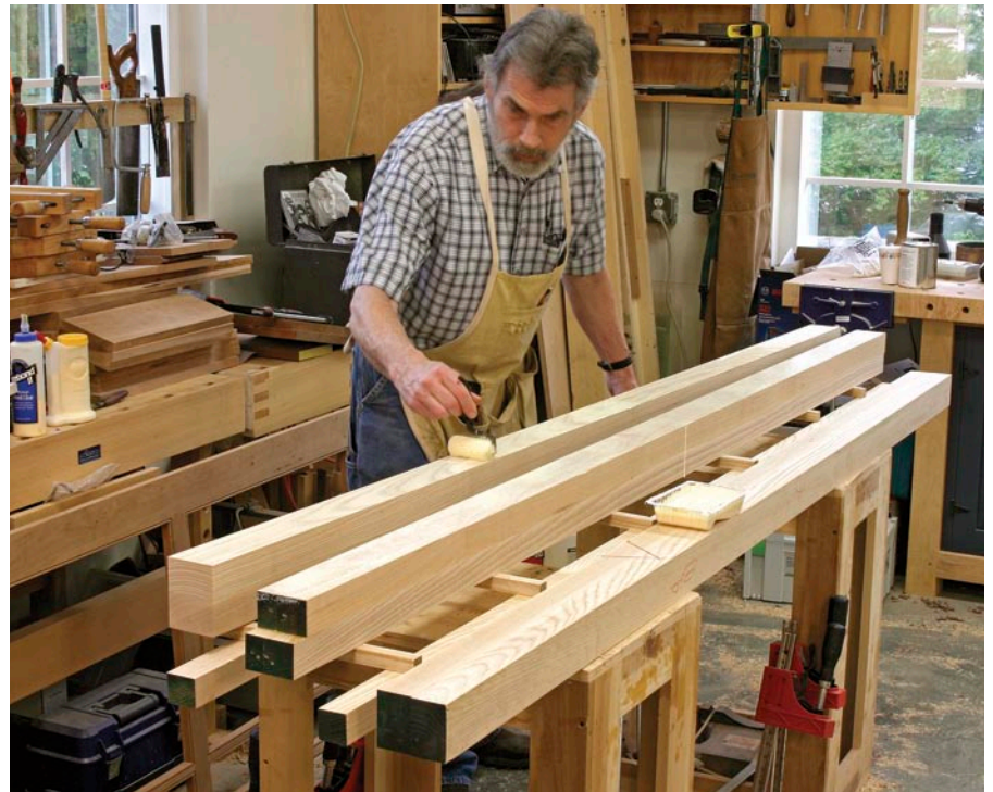
Spread with speed. A disposable paint roller applies an even coat of yellow glue quickly. Apply the glue to one side of the lamination only. Doing both sides wastes time and glue.
