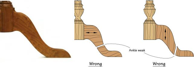
The wood grain in the legs of this pedestal table runs parallel to the longest dimension, making the legs as strong as possible. Were the grain to run parallel or perpendicular to the pedestal, the legs would be weakest at their narrowest point, the ankles.
