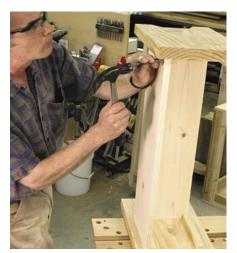
Planning a logical sequence for assembling the parts is important. I attached the front and bottom together and glued and nailed them to the ends as a single unit.
