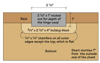
Plan detail of hinge buildup
